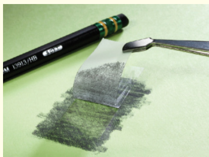
How to obtain a Nobel Prize: peeling off graphene from graphite using Scotch tape.
